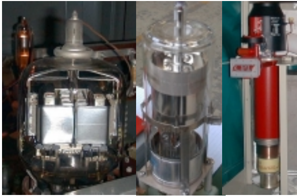
FIG. 1. Different kinds of electron valves, used in radar facilities
